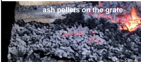
disintegrated granular ash after de-ashing with a robust screw
